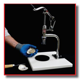
**Step Three** - As the blade penetrates the seam rotate the handle 90° in either direction. This will open the two shell halves and render the muscle accessible.
