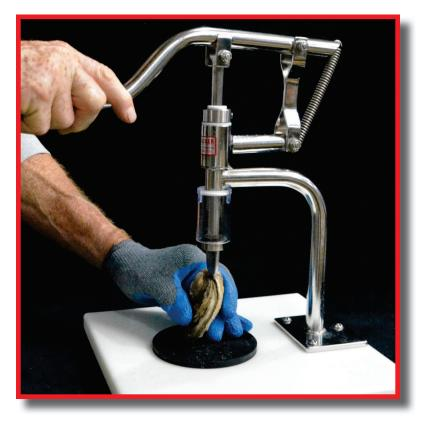
**Step One** - Firmly hold the oyster or shellfish with the heel or hinge pointing upward onto the black rubber pad. While slowly bringing the blade downward, align the seam of the oyster or shellfish directly under the blade. For your safety, use of a protective glove for holding the shell is recommended.
