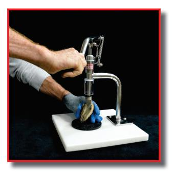
**Step Two -** While still holding the oyster or shellfish with one hand, work the blade into the seam by simultaneously applying downward pressure and moving the handle back and forth in short side-to-side strokes. Technique is more effective than brute force in this procedure. This action will allow the blade to penetrate the seam.
